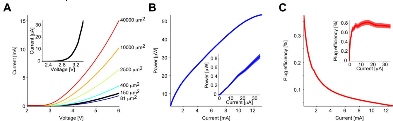
**Figure S1. Full range characterization of the LEDs, related to Figure 3. (A)** Current versus voltage characteristics of various LED sizes (inset correspond to the low-bias characterization of the 150- $\mu\text{m}^2$  LED used in the actual  $\mu\text{LED}$  probes, cf. **Figure 3A**). **(B)** Current versus power. **(C)** Current versus plug efficiency.
