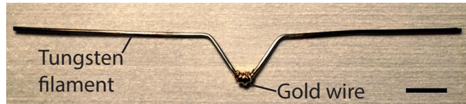
Figure 2: Image of tungsten wire filament prepared with gold wire. Scale bar is 10 mm.
