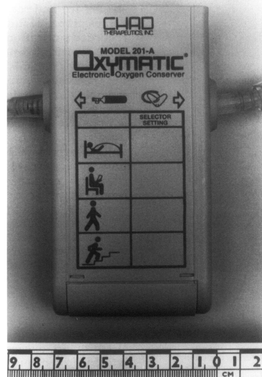
Figure 1 The Chad Oxymatic demand oxygen delivery device.
