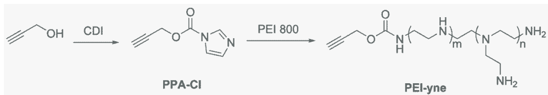
Supplementary Figure 1. Synthesis of PEI-yne. First, propargyl alcohol was reacted with 1,1'-carbonyldiimidazole (CDI) at room temperature to obtain the propargyl ester of carbonylimidazole (PPA-CI). Then, polyethylenimine (PEI, Mw 800 Da) was reacted with PPA-CI to synthesize PEI-yne.
