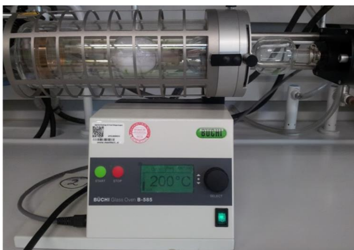
Figure S1. Photograph of Kugelrohr vessel filled with substrate and zeolite.
