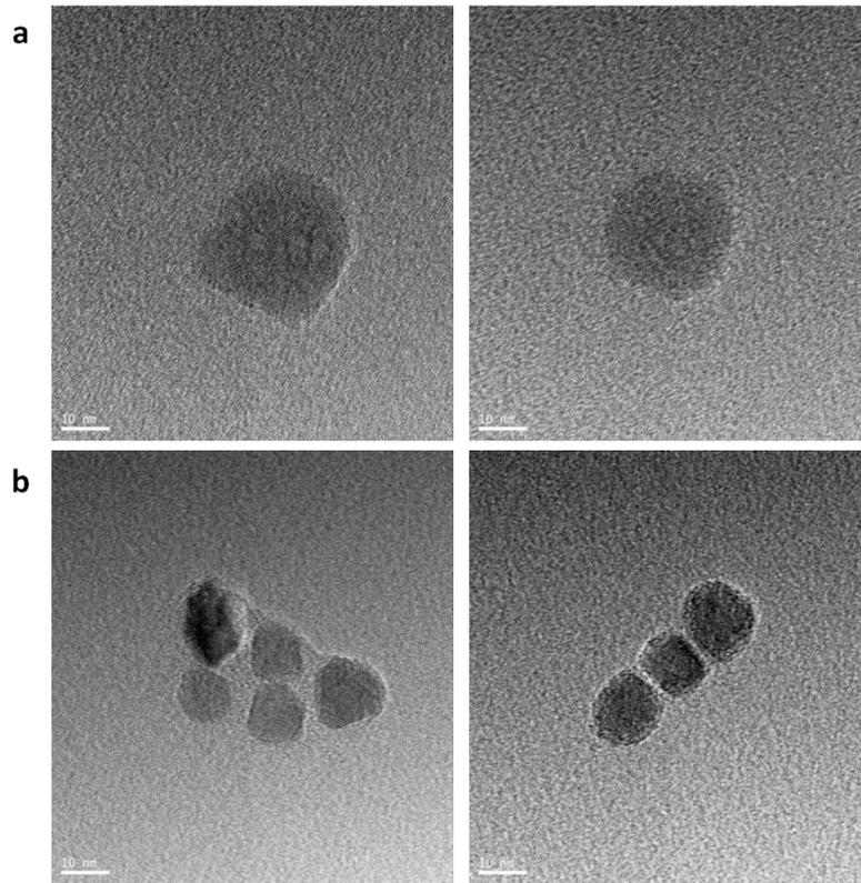
**Supplementary Figure 2.** Transmission electron microscopy (TEM) images of the magnetic nanoparticles before (a) and after (b) conjugation with ASODN.
