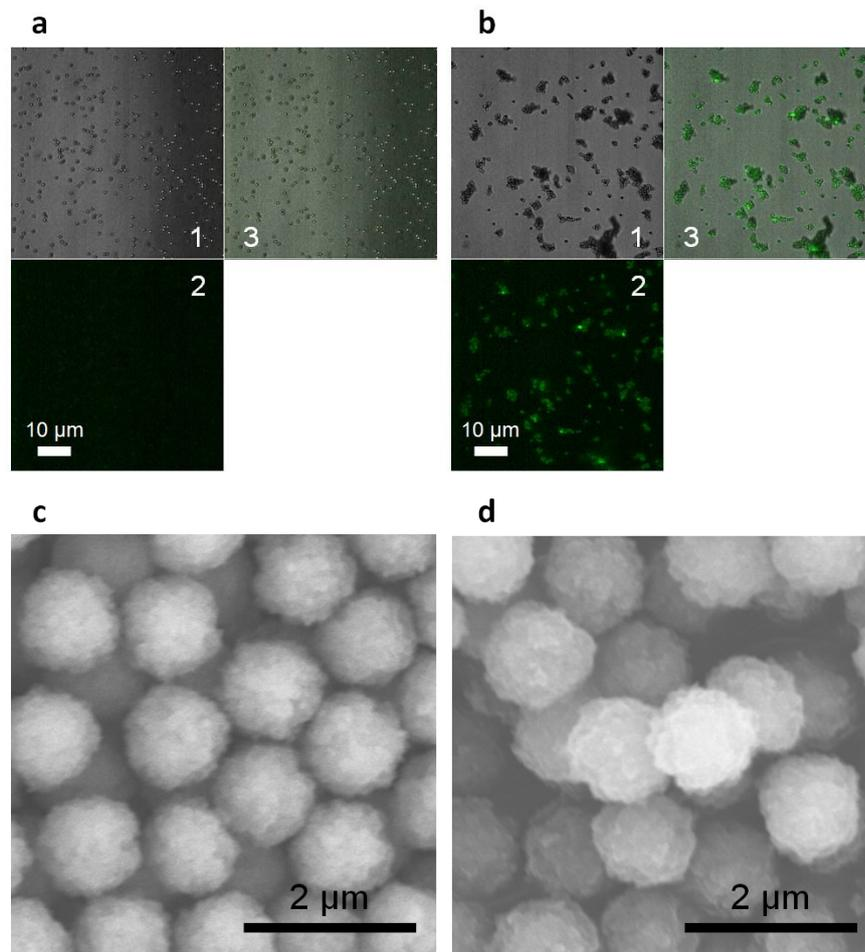
**Supplementary Figure 1.** Confocal laser microscopic images (a, b) and scanning electron microscope (SEM) images (c, d) of magnetic microparticles (1 $\mu$ m) before (a, c) and after (b, d) conjugation with ASODN labelled with FAM and amine at 5'- and 3'-end, respectively. 1, Optical images of the 5 microparticles; 2, FAM fluorescence on the microparticles; 3, merged images of 1 and 2.
