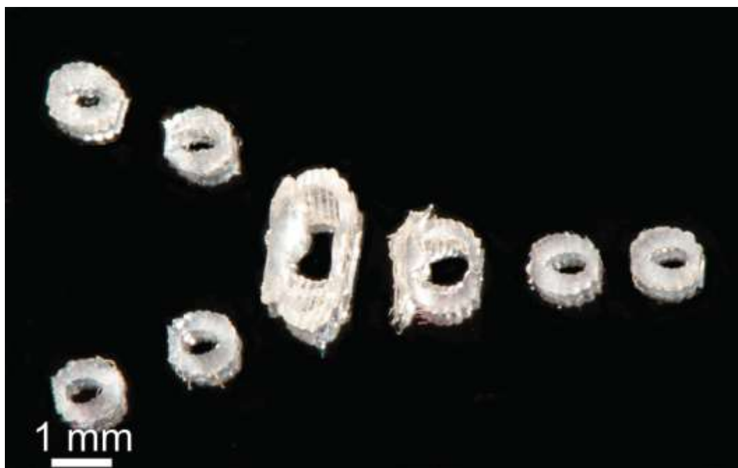
Figure S10. Cross-sectional images of a 3D printed nerve guide at various positions along its length ( L = 10 mm; positions from left to right correspond to L , 0.75L , distal bifurcation region, proximal bifurcation region, 0.25L , and 0 mm).
