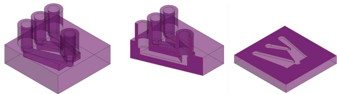
**Supplementary Figure 8 Device configuration for PtNP synthesis.** Rendering of the device geometry used for the synthesis of PtNPs. It contains one inlet for the continuous and two inlets for the dispersed phases and one outlet. Each port accepts OD = 1/16 inch tubing.
