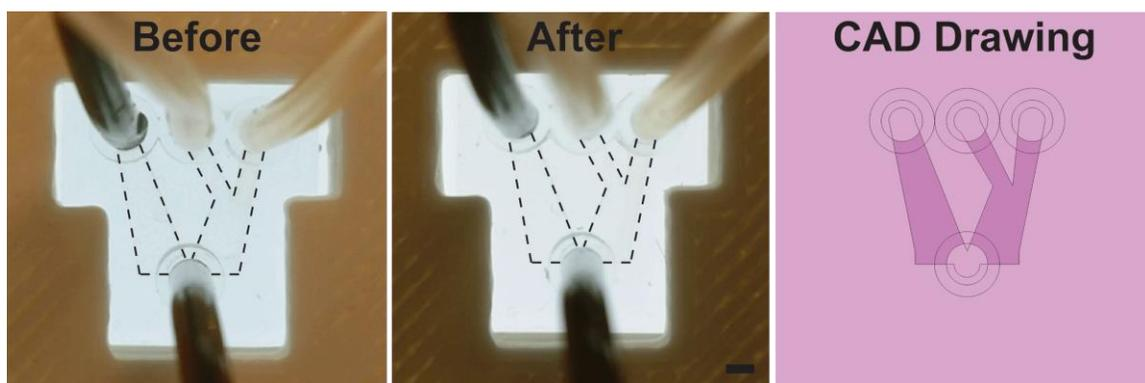
**Supplementary Figure 9 Device resistance to fouling.** Top down view of the droplet generating device from Supplementary Figure 8. It is held in place by a custom clamp. The droplet generating device remains visually unchanged after running the PtNP precursors. The CAD drawing shows the top-down view of the device. Scale bar is the same for all images and represents 1 mm.
