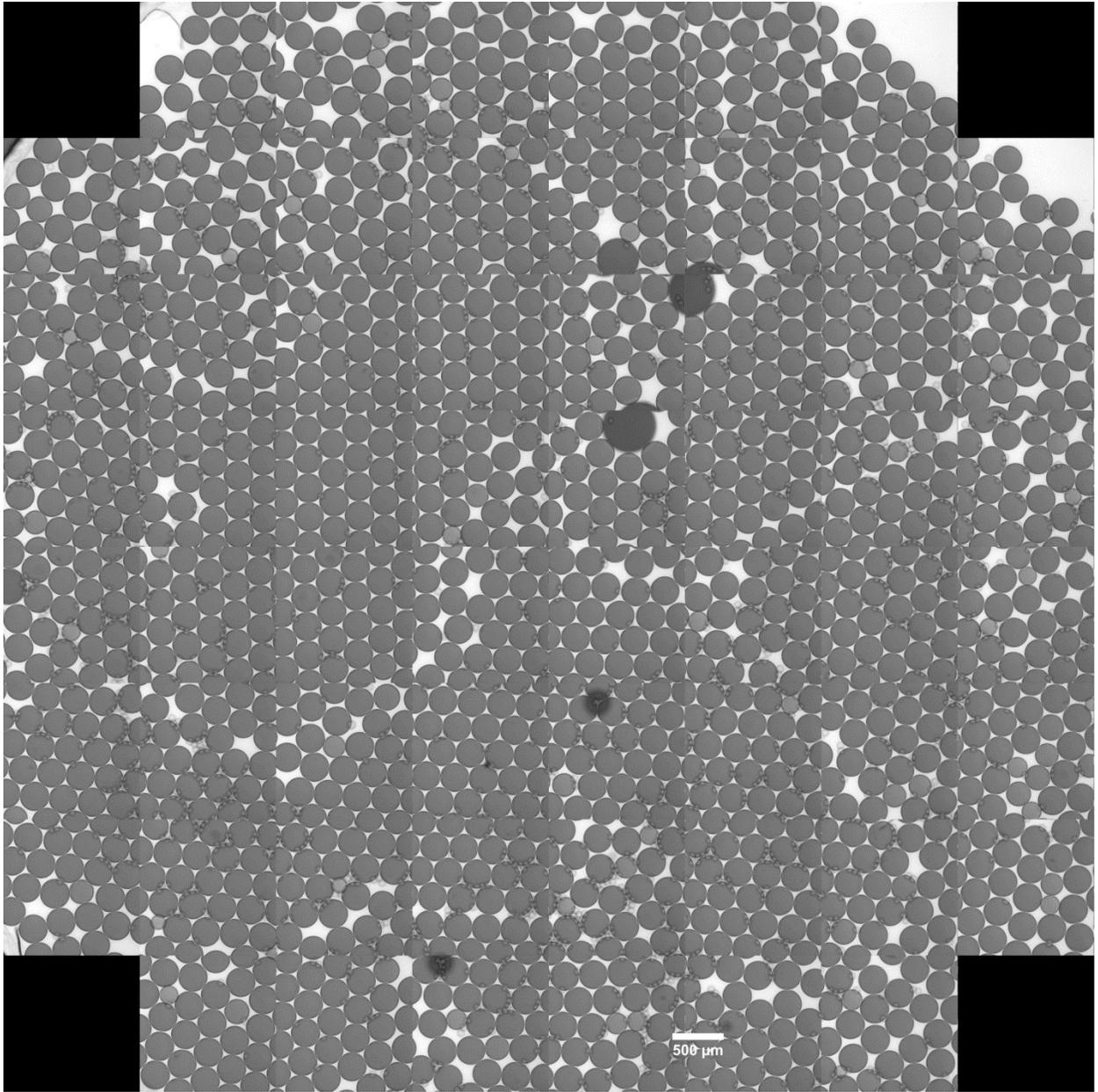
**Supplementary Figure 2 Droplet images.** 60 micrographs of droplets produced using PEEK tubing in the outlet (ID = 254  $\mu\text{m}$ ). Scale bar represents 500  $\mu\text{m}$ .
