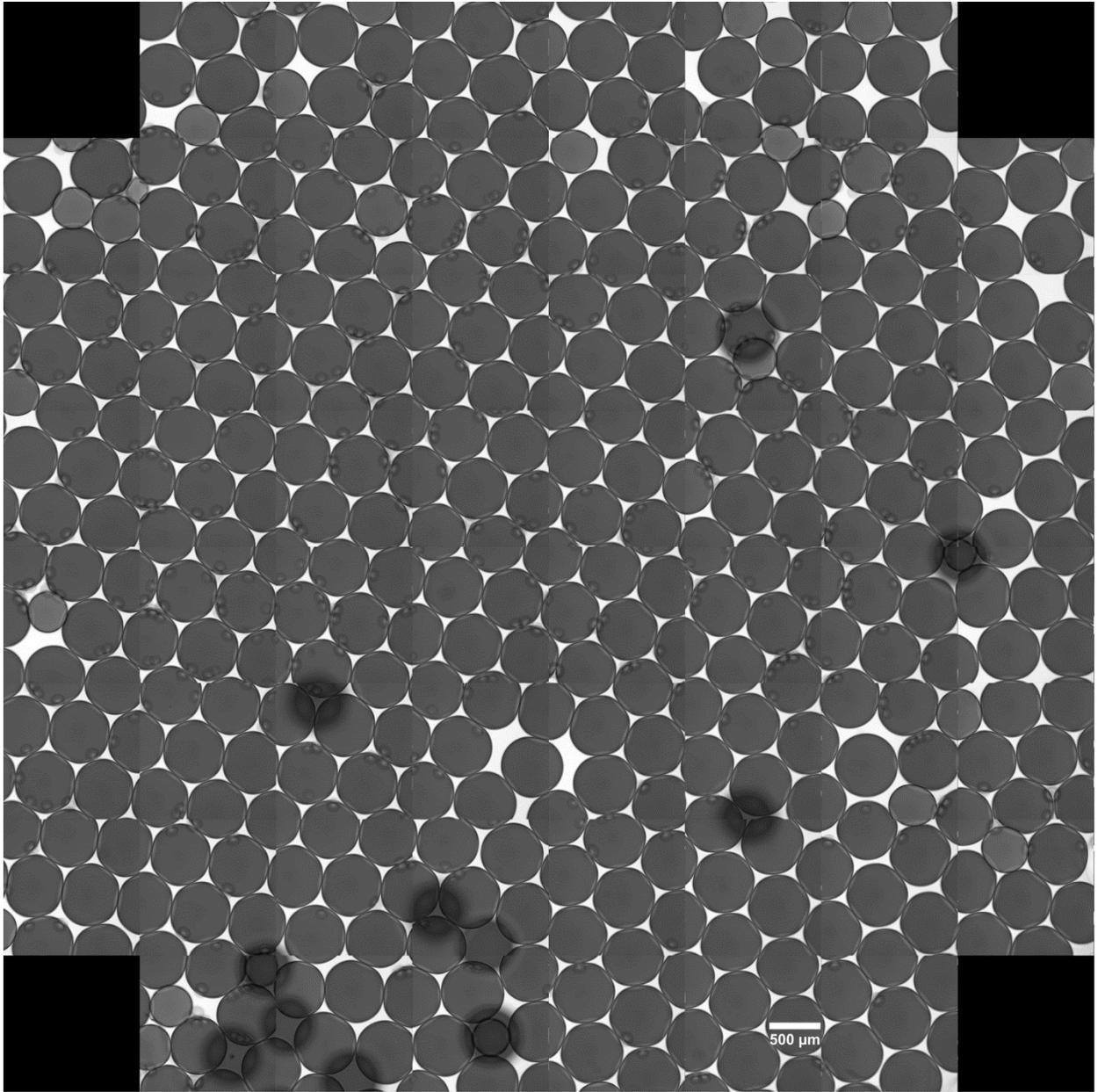
**Supplementary Figure 3 Droplet images.** 60 micrographs of droplets produced using PEEK tubing in the outlet (ID = 508  $\mu\text{m}$ ). Scale bar represents 500  $\mu\text{m}$ .
