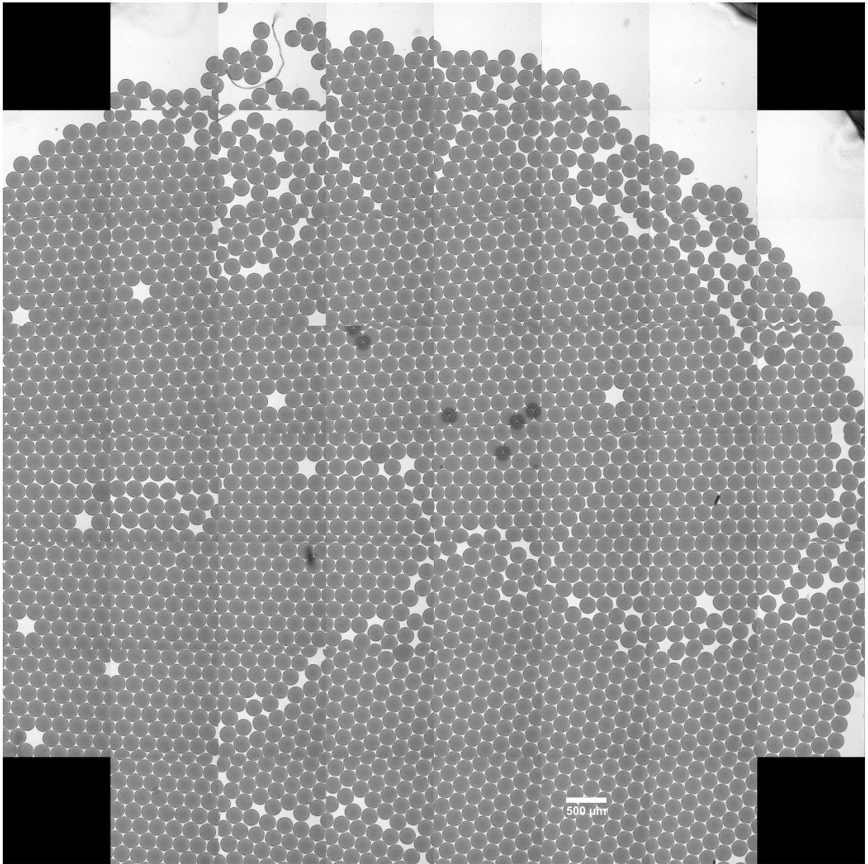
**Supplementary Figure 1 Droplet images.** 60 micrographs of droplets produced using PEEK tubing in the outlet (ID = 178  $\mu\text{m}$ ). Scale bar represents 500  $\mu\text{m}$ .
