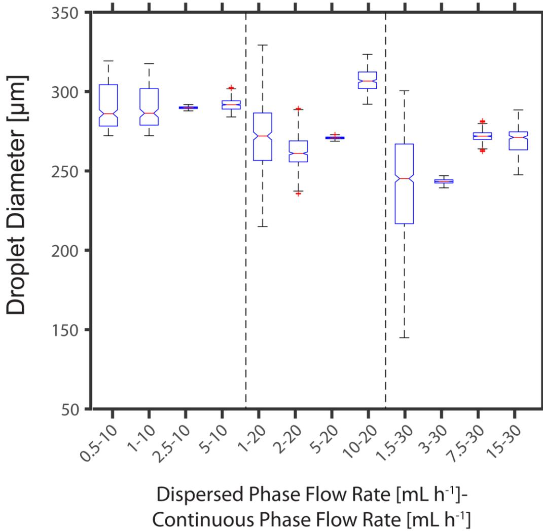
**Supplementary Figure 5 Statistics for viscous droplets.** Boxplot of glycerol droplets formed using the 3D droplet generator and PEEK outlet tubing (ID = 254 μm).
