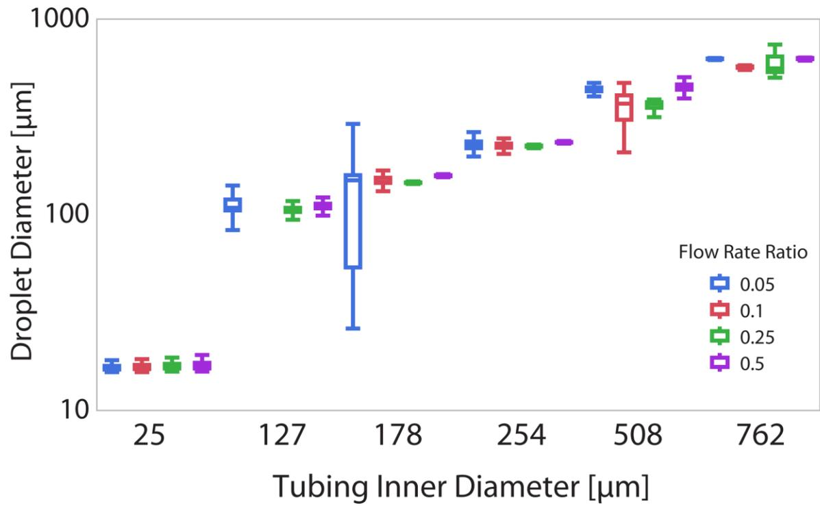
**Supplementary Figure 4 Statistics for droplet sizes.** Boxplot of the droplet sizes produced for different sizes of outlet tubing and different flow rate ratios.
