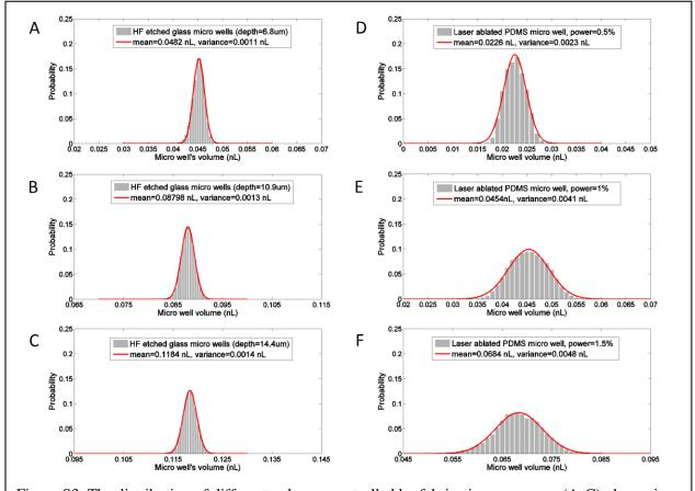
Figure S3. The distribution of different volumes controlled by fabrication processes. (A-C) glass micro wells with increasing HF etching time, giving depths of 6.8, 10.9 and 14.4 µm, respectively. Depths are measured by stylus profilometry. (D-F) PDMS micro wells with increasing laser power at 0.5, 1 and 1.5% respectively.
