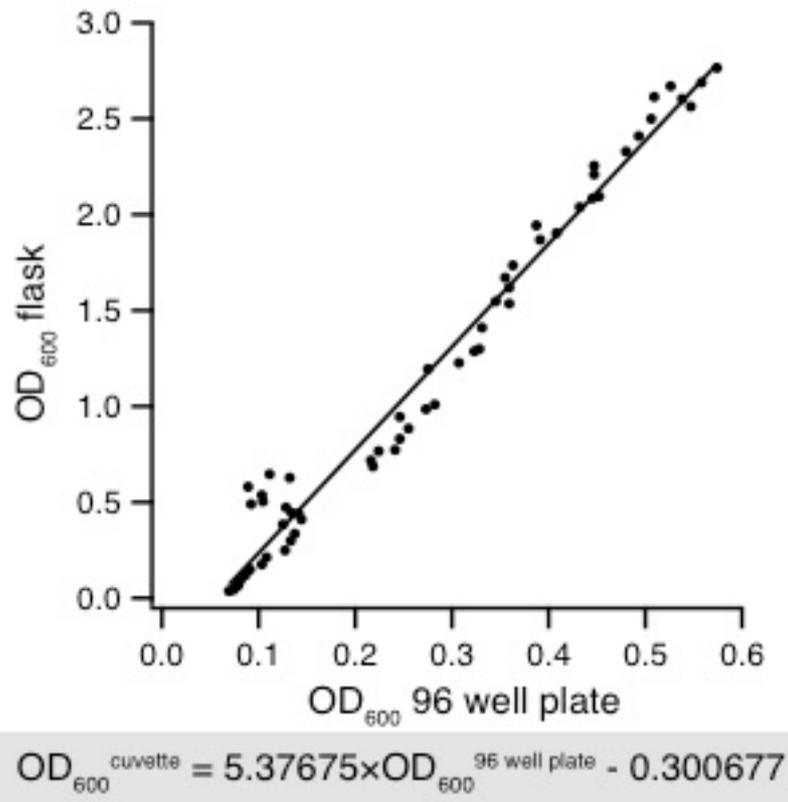
**Supplementary Figure 5 | Calibration curve for conversion of OD<sub>600</sub> readings obtained using a 96-well plate reader and a spectrophotometer.**
