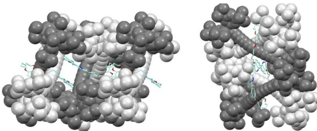
**Figure S26.** The crystal packing the [3]rotaxane **(2c)<sub>2</sub>·M1** viewed down to crystallographic *a* (left) and *b* axes. The A and B chains of hexayne are colored differently. Hydrogen atoms are omitted for clarity.
