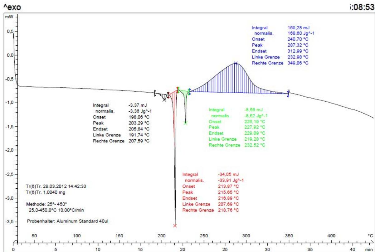
**Figure S27.** DSC trace of **2c·M1**. We assign the peak at 216 °C to the melting of the compound (from measuring the melting points by conventional method). The peaks at 203 and 228 °C are attributed to the phase transitions.
