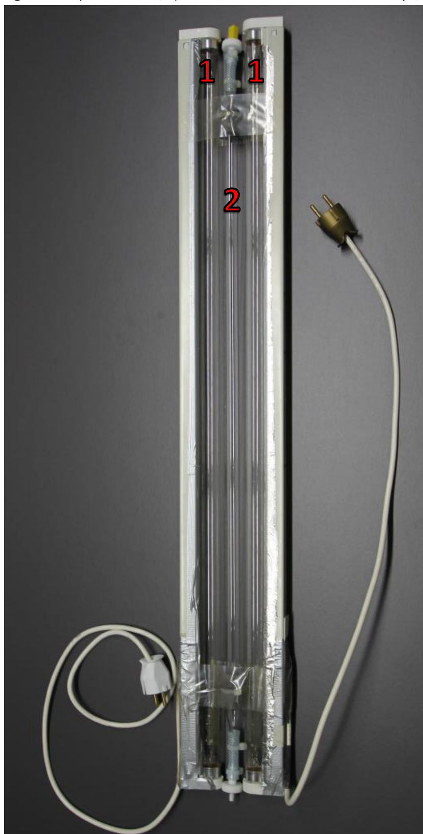
Fig. S1 Flow photoreactor; 1) 55W OSRAM HNS 90 cm T8 OFR lamps; 2) Quartz tube
