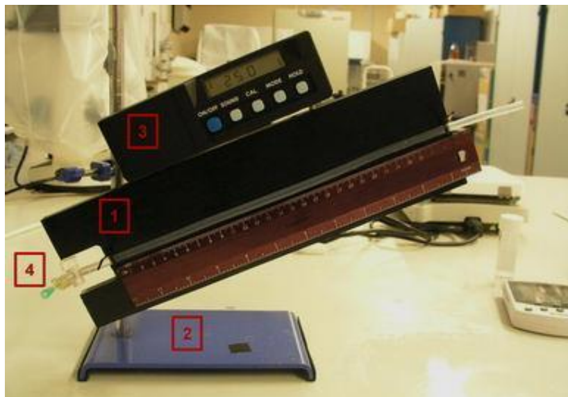
Figure S2.1 Photograph of the experimental set-up. PTFE tubing in a platform (1) stabilised within a manifold (2). Platform angle was measured by a digital inclinometer (3). A three-way stopcock at the lower end of the tube allowed sequential tube filling, foam injection and tube flushing (4). (Taken from Ref. [1])
