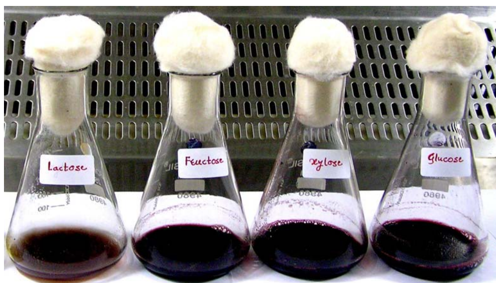
Figure S1. Production of bikaverin in shake flasks by Fusarium fujikuroi Mut-4 using different carbon sources
