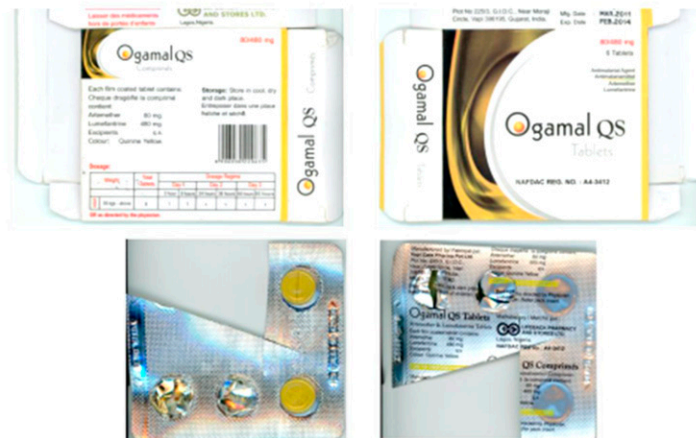
SUPPLEMENTAL FIGURE A8. Liquid chromatography mass spectrometry analysis of artemether/lumefantrine (AM/LUM) Ogamal QS tablet reveals similar degradation products to Coartem ® AM/LUM tablets artificially degraded. Examination of the packaging revealed a sticky residue inside the blister pack, and tablets were discolored.
