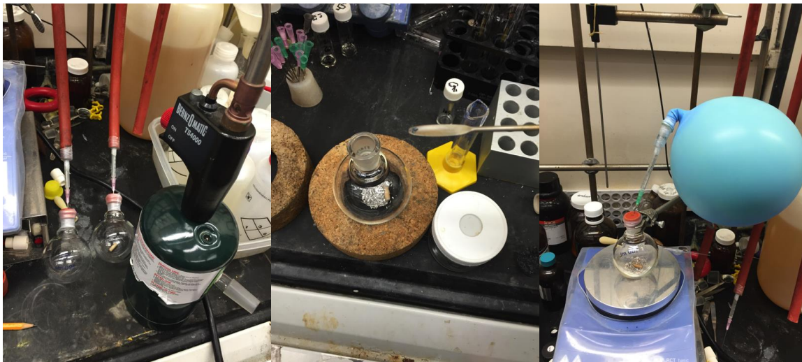
(Left) Two round-bottom flasks under vacuum after flame-drying with a blowtorch. (Center) After cooling, one flask was charged with Mg turnings and I 2 . (Right) Flask containing Mg and I 2 under Ar inert atmosphere.
