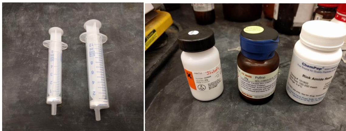
(Left) Solid-phase reaction vessels purchased from Torviq. (Right) General coupling reagents (HATU and PyBOP) and ChemPep Rink amide resin.
