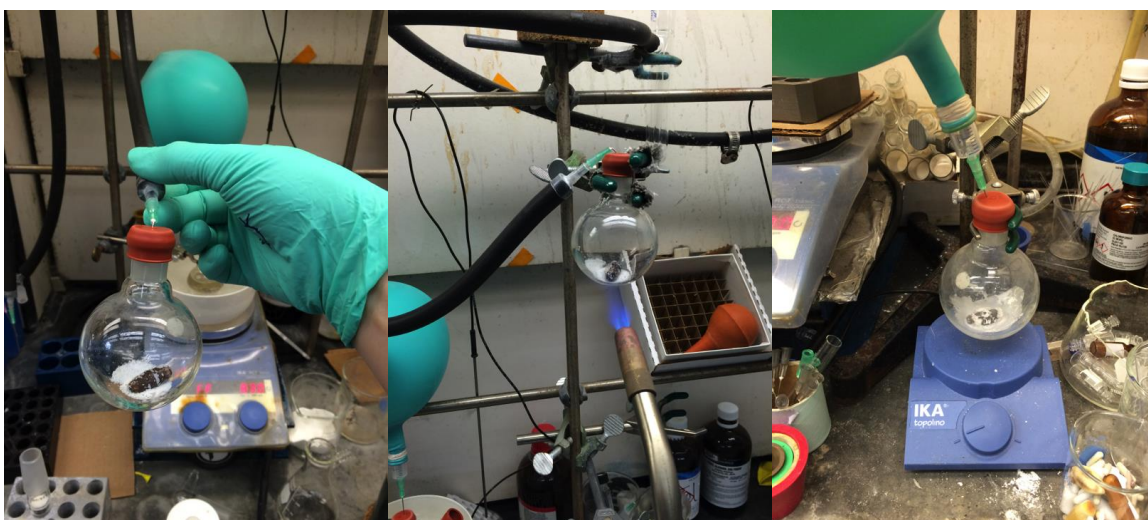
(Left) ZnCl 2 . (Center) Flame-drying ZnCl 2 until the solid melts. (Right) After flame-drying, under inert Ar atmosphere.
