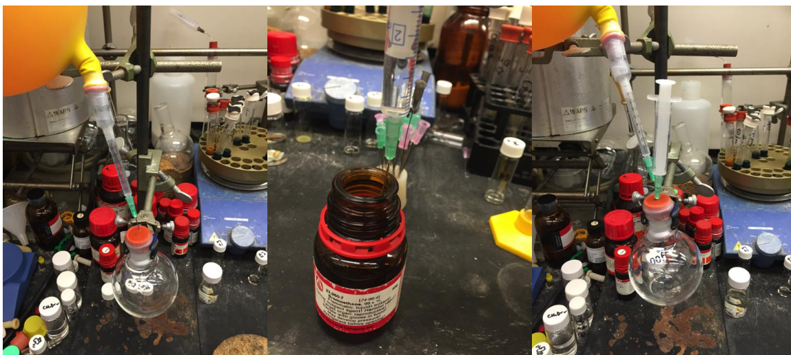
(Left) Round-bottom flask under Ar inert atmosphere. (Center) EtBr is taken up into a syringe. (Right) EtBr is added to the flask.
