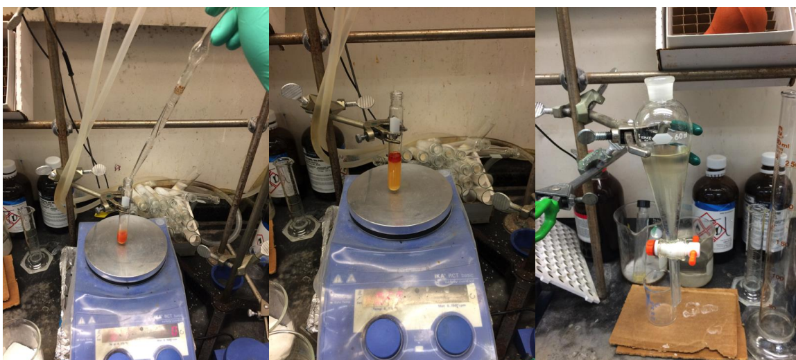
(Left) Quench with half-saturated \text{NH}_4\text{Cl} (aq). (Center) After quench. (Right) Quenched reaction mixture was transferred to a separatory funnel and extracted with EtOAc, dried, and concentrated.
