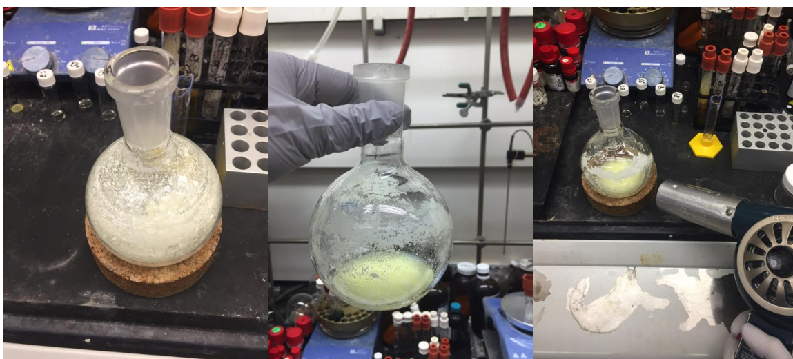
(Left) Product after column chromatography. (Center) After addition of \text{CH}_2\text{Cl}_2 . (Right) The mixture is heated with a heat gun until all material solubilizes.
