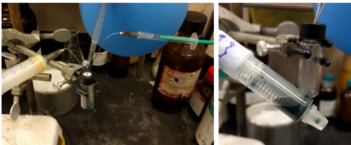
(Left) A syringe containing the diethylzinc solution (right-hand syringe) is pierced into the septum of the small reaction vial containing the DMF solution of ligand and nickel catalyst; the resin-bound peptide (left-hand syringe) is poised for addition of the nickel solution, followed immediately by the addition of the dialkylzinc solution. (Right) Capped, resin-bound peptide following addition of nickel and dialkylzinc; note that the dark green color emerges within a few seconds of addition of both reagents to the resin.
