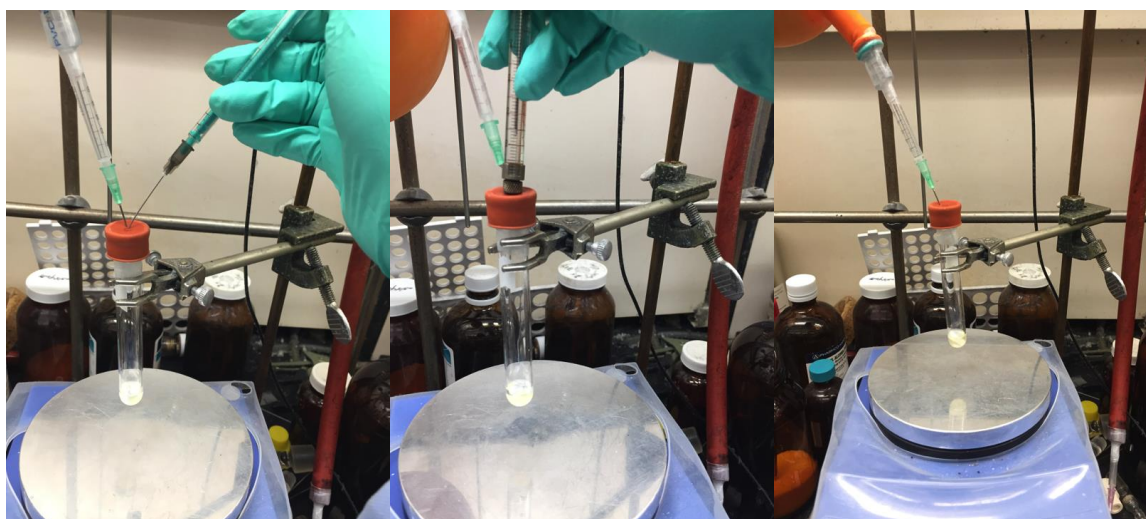
(Left) Addition of DMF. (Center) Addition of Et 3 N. (Right) After addition of Et 3 N, mixture becomes homogenous.
