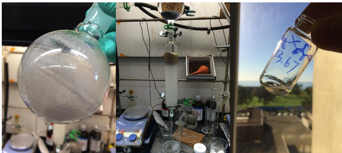
(Left) Crude product. (Center) Purification by column chromatography. (Right) Pure product.
