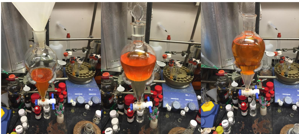
(Left) Quenched reaction mixture was transferred to a separatory funnel. (Center) Extraction with \text{Et}_2\text{O} . (Right) Brine wash.
