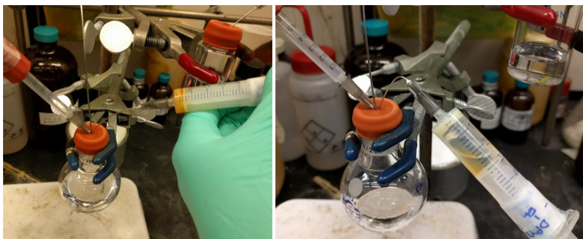
(Left) Following expulsion of the activation solution, the resin-bound peptide is washed with dry DMF (5 x 3 mL), dry MeOH (5 x 3 mL) and dry DMF (5 x 3 mL). (Right) Close-up of resin washing with DMF; following brief mixing with the resin, the washing solutions are expelled into the waste.
