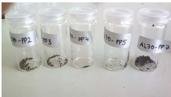
Figure S3. NPs purified by repeated precipitation and magnetic decantation. As the purification proceeds, the color of the sample changes to a darker brown which is attributed to the removal of free NDA-PEG.
