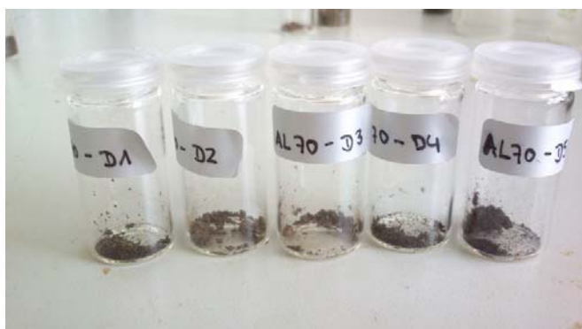
Figure S2. Dialyzed NP dispersions after 1h, 2h, 6,5h, 24h and 48h. The color changes from brown to black due to removal of free PEG and results in almost black samples, indicating that also bound NDA-PEG has been ripped off the surface and leaving almost bare cores.
