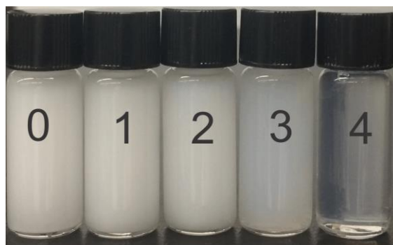
Supplementary Figure 14: Photograph of T-undec. InFroMs in hypertonic saline. T-undec InFroMs were prepared in 10 % F127 (w/v) with different NaCl concentrations (0, 1, 2, 3, 4 M as indicated by the numbers in the photo). Results are representative of 3 independent trials.
