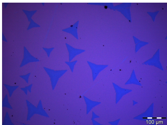
Figure S1: Optical image of CVD grown MoS 2 flakes on SiO 2 .
