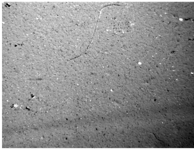
Figure S5: Topographical Image of Co/Ni Multilayered film under saturating magnetic field.
