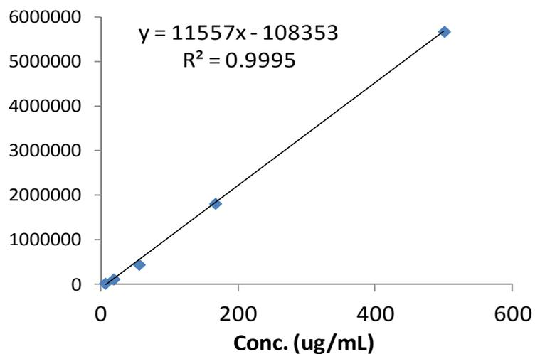
**Figure S3. Standard curve of IGF1 ligand by HPLC method with UV detection at 280 nm.** It showed a good linear range for IGF1 concentration from 15.6 to 500  $\mu\text{g/mL}$  with  $R^2 = 0.9995$ . The injection volume was 25  $\mu\text{L}$ .
