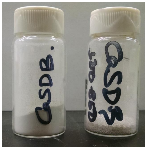
Supplementary Figure 28. Pallet (500-850 \mu\text{m} size) of SBMOF-1 (right), made by a mechanical sieving process (CaSDB = SBMOF-1)
