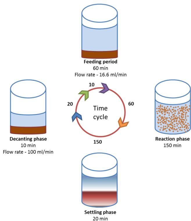
**Figure S8** A schematic of the operation stages in the laboratory SBR consisting of feeding, reaction period with mixing with 5% CO<sub>2</sub> + 95% Argon gas, settling period and decanting period. Figure S8 was created by Samik Bagchi.
