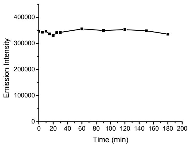
**Figure S17.** The upconversion emission at 542 nm of dye-sensitized  $\beta$ -NaYF<sub>4</sub>:20%Yb,2%Er/ $\beta$ -NaYF<sub>4</sub>, 10%Yb core/Yb<sup>3+</sup>-shell UCNPs PMMA film soaked in PBS over the course of three hours. (2 W/cm<sup>2</sup> 800 nm CW laser).
