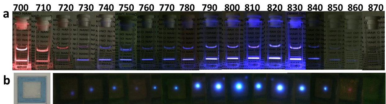
Figure S39. Blue upconversion emissions from IR-808 and IR-820 co-sensitized ( \text{NaYbF}_4: \text{Tm}^{3+} 0.5%)@ \text{NaYF}_4: \text{Nd}^{3+} core/shell nanoparticles (a) dispersed in DMF solvent (1 wt%) and (b) in a polystyrene film (~30 wt%). The photographic image of home-made IR card is displayed on the left corner in b.
