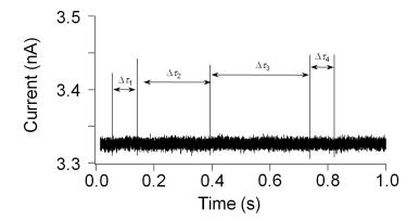
**Figure S2**. A portion of a 60.85 sec *i-t* trace recording 570-nm-radius microgel particle translocation events through a 433-nm-radius GNM. The experiment was performed in a 10 mM KCl, 1 mM PBS (pH 7) solution with an applied voltage and pressure of +0.1 V and -50 mmHg, respectively (internal vs. external).
