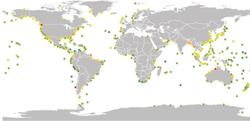
Supplementary Fig. 2: GTSR performance over 1980-2011 as the RMSE (m) for a , surge levels, which are simulated by forcing GSTSM with meteorological fields from ERA-Interim 4 ; and b , tidal levels modelled with FES2012 3 .
