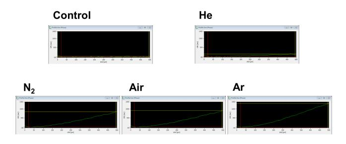
Line profile (side view) of a cantilever observed by DHM under a flow of different gases.
