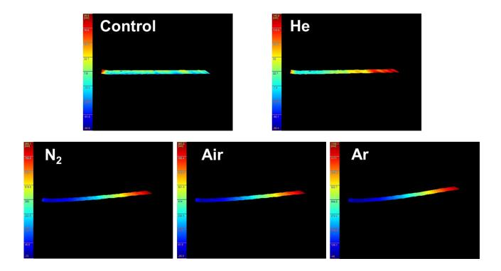
3D images of a cantilever observed by DHM under a flow of different gases.
