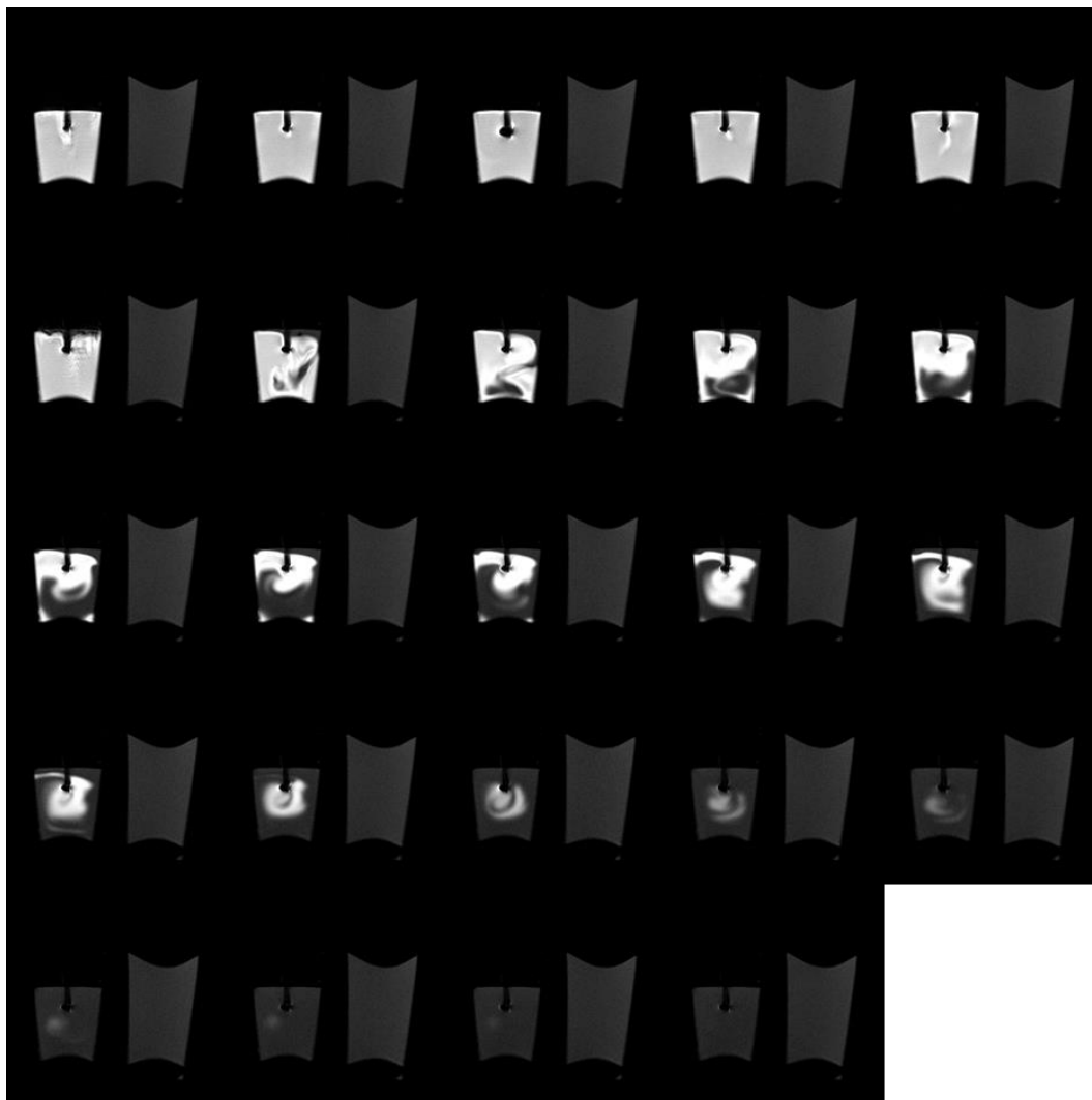
Figure S9. T_1w images acquired of the forced oxidation of \text{Eu}^{2+}\text{DOTA}(\text{gly})_4 (left) with \text{H}_2\text{O} as a reference (right) at 2.5 minute intervals.
