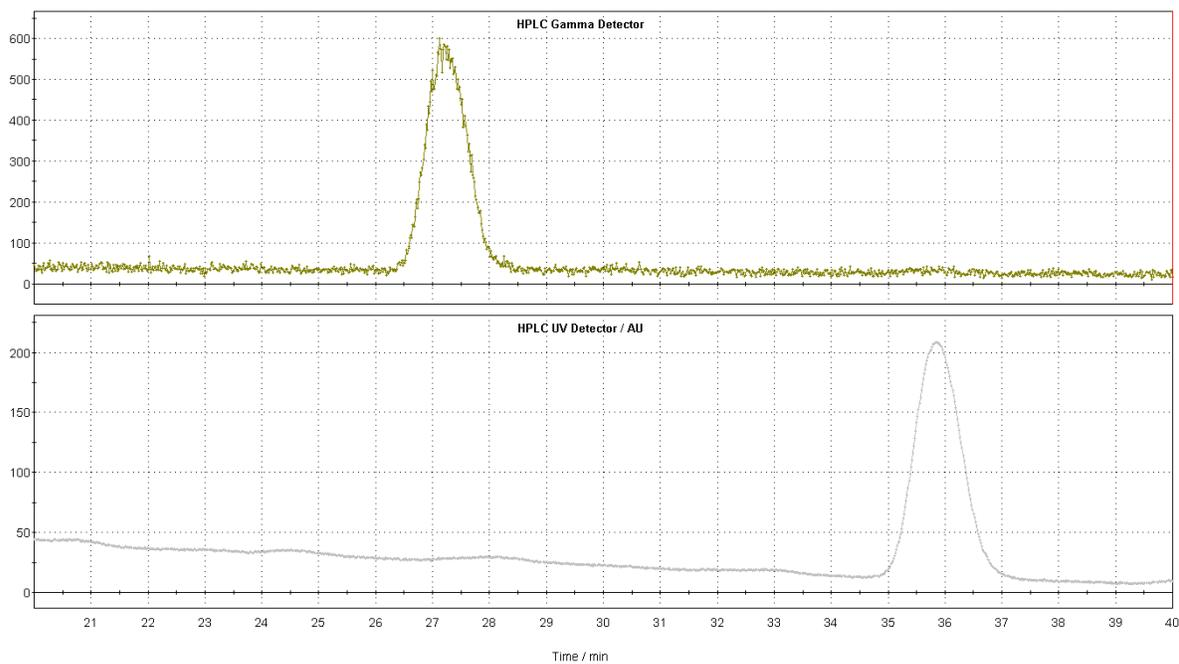
Typical Analytical HPLC trace for [<sup>18</sup>F]FL2-b(black; left y-axis) quality control. Blue overlay is FL2-b reference standard(right y- axis; offset +10mVolts); pink overlay is FL2-b precursor(right y- axis; offset +15 mVolts):
