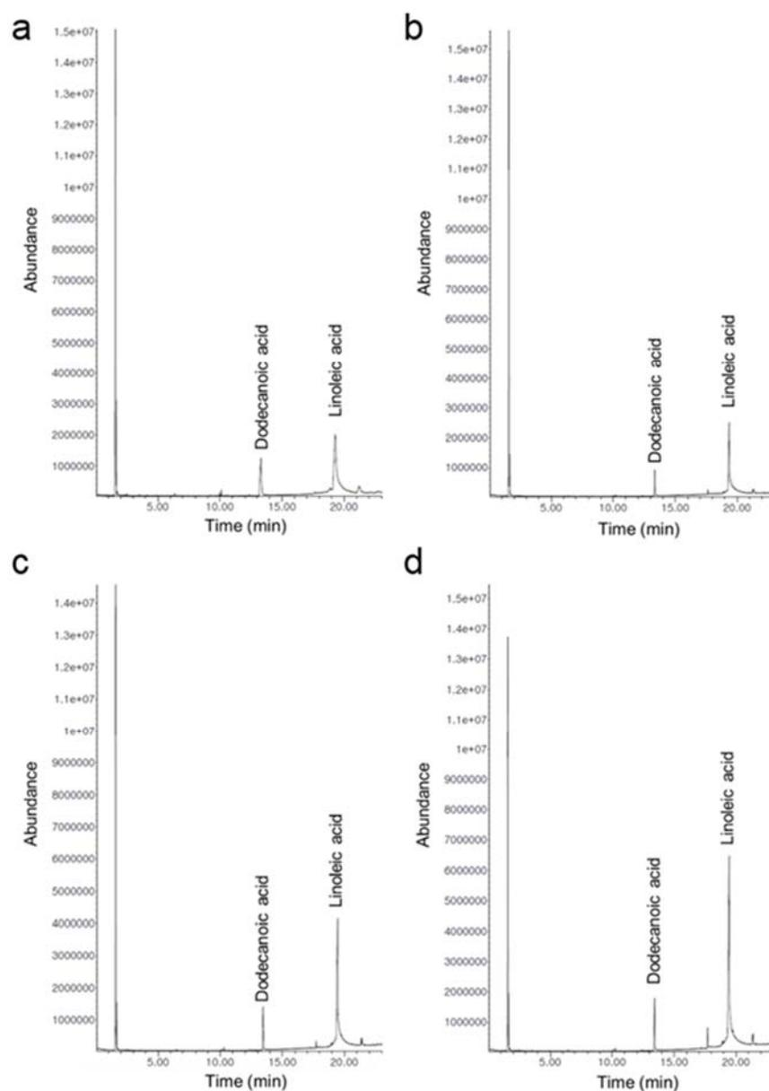
**Figure S1. Gas chromatography analysis of sesame oil incubated with cell-free synthesized PLA1.** 0 (a), 10 (b), 20 (c) and 30 (d)  $\mu\text{g}$  of cell-free synthesized PLA1 were added to 10 mL of crude sesame oil. After 12 h incubation, samples were taken and analyzed by gas chromatography as described in Methods.
