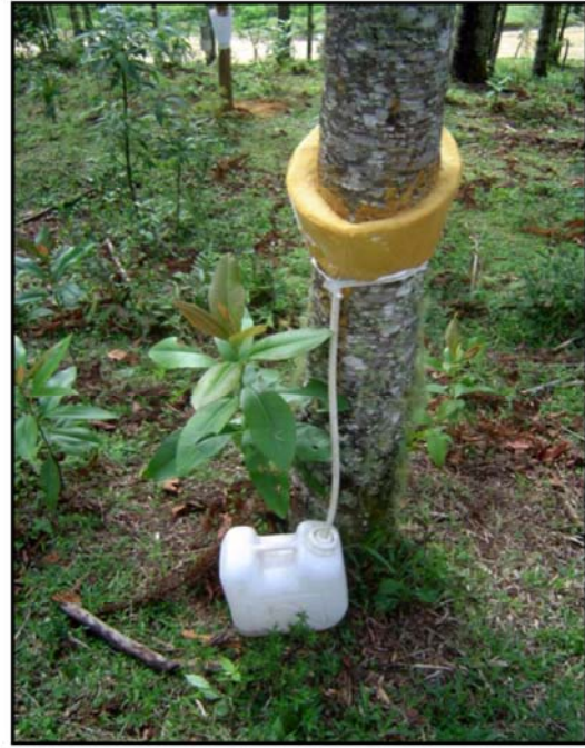
Figure S2: Rain measuring devices. Funnel precipitation gauge used to collect gross rainfall and throughfall (a) and polyurethane collector used to collect the stemflow (b).
