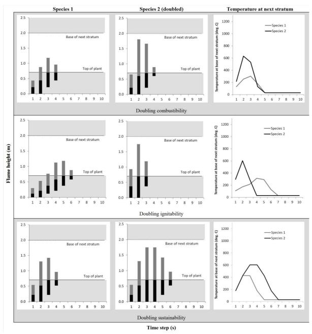
The effect of doubling different flammability metrics on flame height, flame duration and the temperature to which the base of next stratum is exposed. In each case, all metrics are held constant except for the one being examined. Shaded areas show plant strata, the dark bars show the part of the plant that is burning in that time step, and the lighter bars show the flame extending from the burning foliage.
