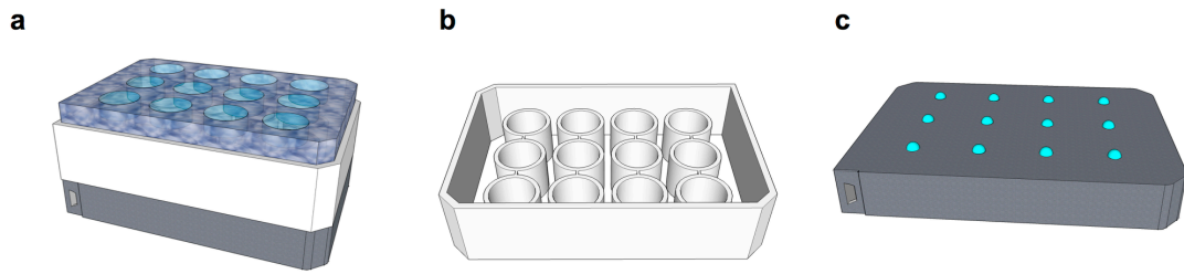
Supplementary Figure S1: 12-LED Blue Light Source setup. (a) The 12-LED blue light source is designed to provide 465nm light for the 12-well culture plate, with adjustable on/off time and light intensity on individual wells. This design incorporates a sandwich structure, where light & circuit enclosure sits at the bottom, followed by a whitespacer in the middle, and a 12-well culture plate on top. (b) The spacer holds and aligns the light & circuit enclosure with the culture in position. The tube structure inside the spacer helps to diffuse and isolate the 12 light channels for individual wells on the plate. (c) Micro controller and LED driver circuit sit inside the bottom casing, with through-hole LEDs mounted directly on top.
