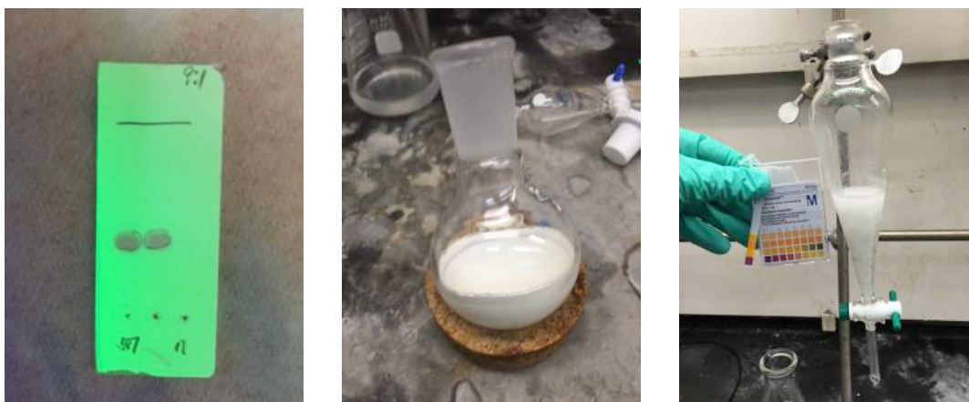
Left: TLC plate of the reaction mixture (left: starting material; center: cross-spot; right: reaction mixture). Center: evaporation to dryness. Right. pH adjusted with 1M HCl in a separating funnel after dissolving with \text{CH}_2\text{Cl}_2 .
