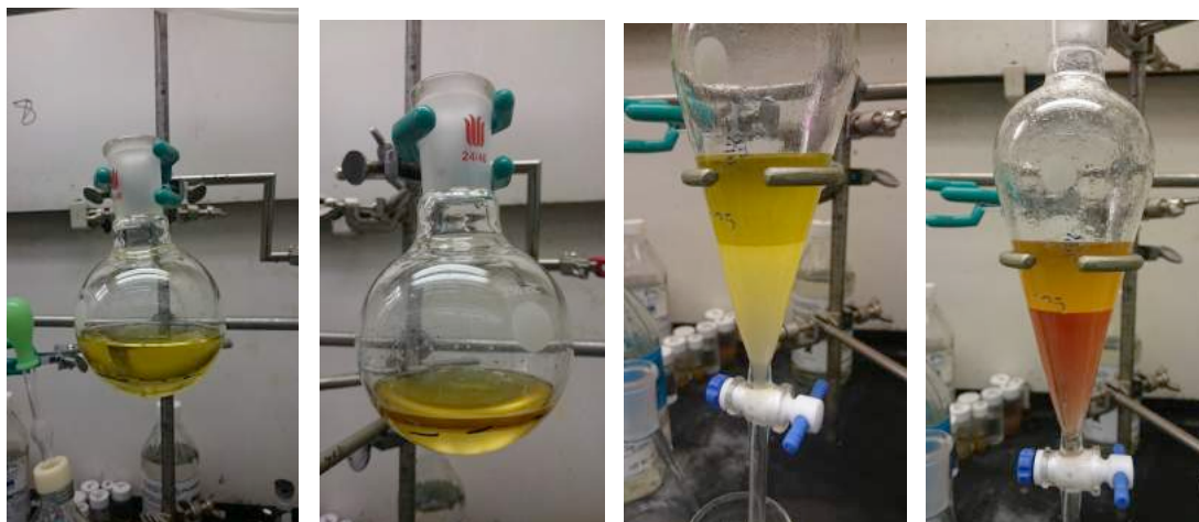
Left: reaction mixture after quench with HCl. Center-left: after removal of THF. Center-right: addition of toluene and extraction. Right: initial wash with water (pH = 0).
