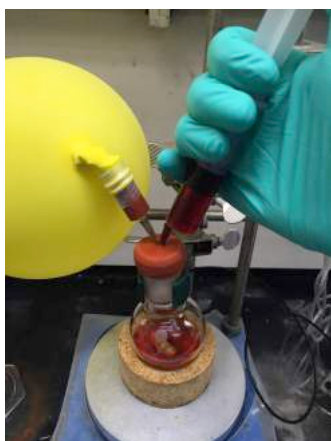
Left: addition of Fe/ligand solution. Center: addition of the organozinc at 0 °C. Right: quench the reaction after 1 h with 1M HCl.
