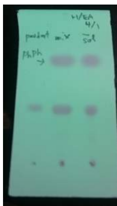
TLC plate (left: pure material; center: cross-spot; right: organic solution after washing).
