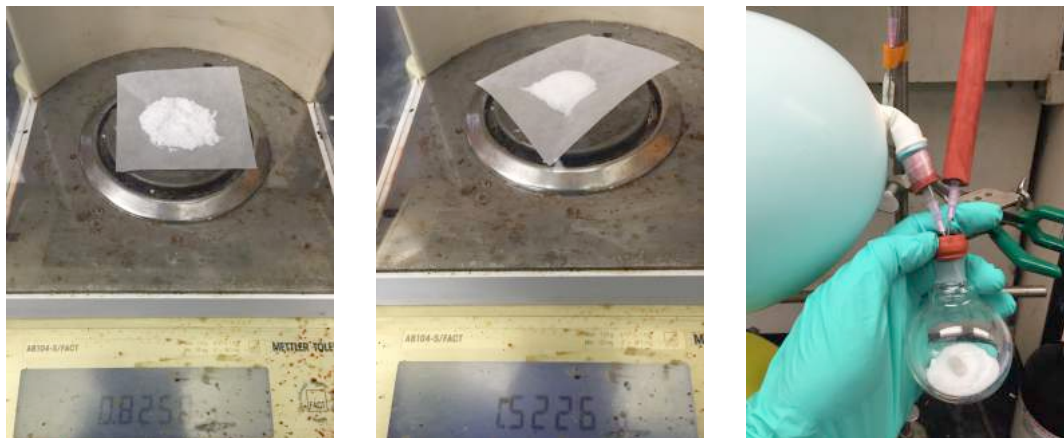
Left: carboxylic acid weight. Center: HATU weight. Right: carboxylic acid and HATU in a flask, evacuated and backfilled with Ar.
