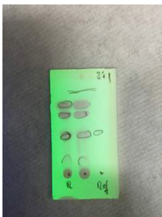
Left: TLC plate of the reaction (left: reaction mixture; center: cross-spot; right: pure material). Center: column chromatography. Right: isolated pure material.
