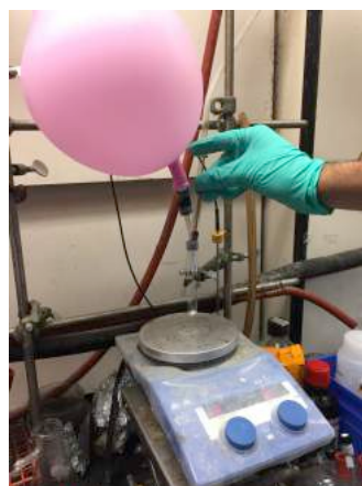
Left: Weighted solids in a culture test tube under Ar. Center: Anhydrous triethylamine utilized. Right: Addition of triethylamine.
