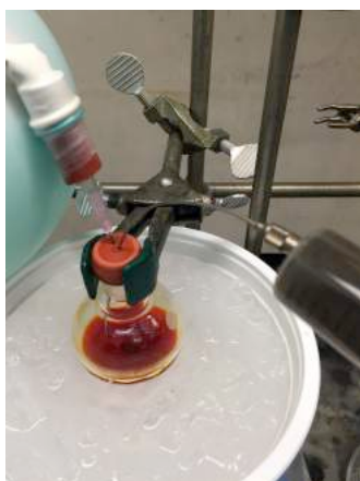
Left: addition of Fe/ligand solution. Center: addition of the organozinc at 0 °C. Right: reaction after 1 h at r.t.
