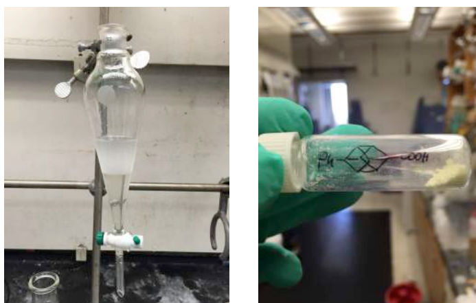
Left: two phases. Right: pure product after evaporation of the organic layer.
