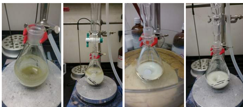
Left: concentration to 10 mL of toluene. Center-left: dropwise addition of 2-PrOH using an addition funnel. Center-right: stirring the system at 50 °C. Right: after cooling down and crystallization.
