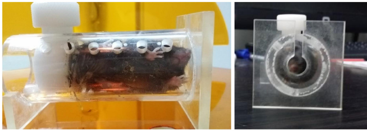
Figure S1. The apparatus of the 24-hour-restraint. The restraint apparatus is a ventilated clear plastic tube (3cm in diameter×10cm). The holes (0.5 cm in diameter) in the head and along the sidewall of the tube enabled air flowing and keep warm as well. Animals could move head and anterior limb, but the body and hindquarters were not able to move or turn around.
