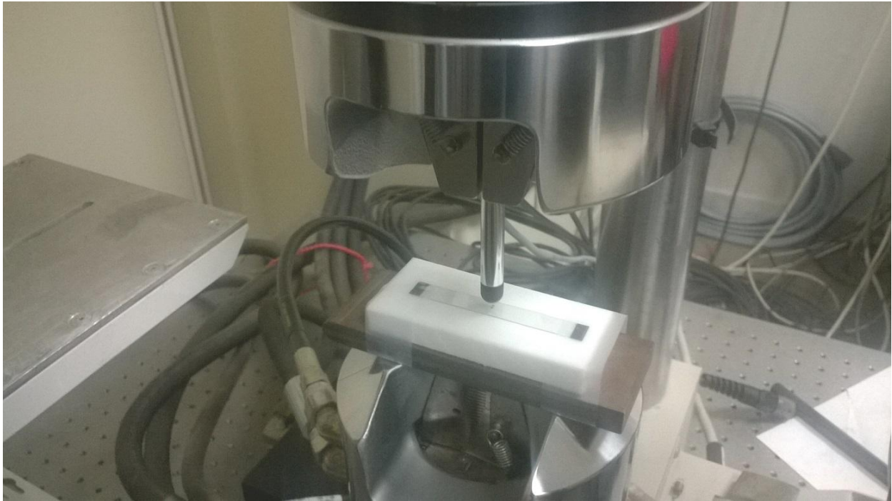
Figure S8. Experimental set-up to simulate the finger force of a typical user via a mobile stylus over a specimen area of 20 \times 20 \mu\text{m}^2 .
