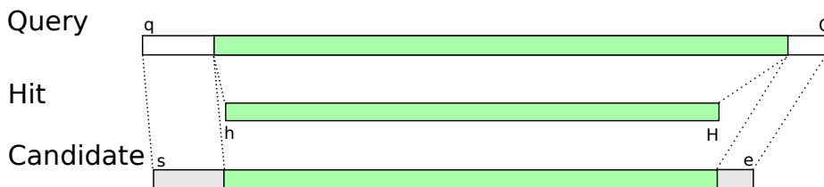
Fig. 3. Extension of BLAST hit and query on the same strand to query length, where h is the start coordinate of the hit, t is the extended start coordinate, q is the start coordinate of the hit on the query, H is the end coordinate of the hit, T is the extended endcoordinate, Q is the end coordinate of the hit on the query, L is the length of the query sequence b is the length of the sequence the hit maps to s is the start coordinate of the extended sequence checked for being within the available coordinates of the hit sequence, E is the end coordinate of the extended sequence checked for being within the available coordinates of the hit sequence
