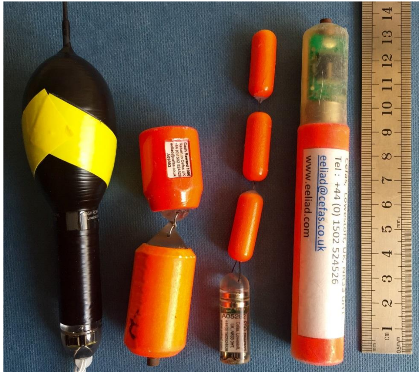
fig. S7. Electronic tag types and attachment technique. (a) Tag types used in the study (from left to right): Microwave Telemetry X-tag, Cefas Technology Ltd pop-off archival tag v2, Cefas Technology Ltd internal drift archival tag and Cefas Technology Ltd pop-off archival tag v1; (b) the ‘Westerberg’ tag attachment method. Eel drawing by Lene Jacobsen (DTU-Aqua).
