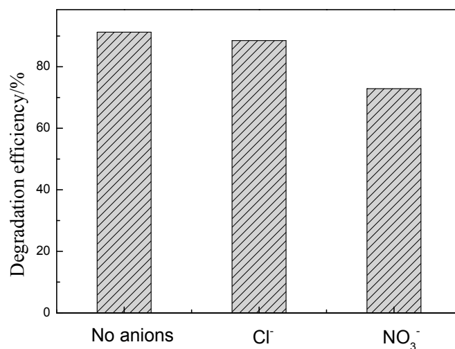
Figure S3. Effect of inorganic anions Cl - and NO 3 - on photocatalytic degradation of benzohydroxamic acid.
