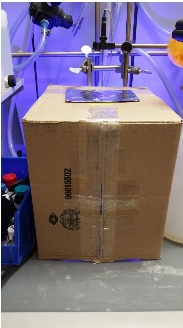
Figure S2. The reaction apparatus during operation. As the LED lamp used for this reaction is a high intensity blue light source, it is suggested that precautions be taken to prevent unnecessary ocular exposure to stray light.
