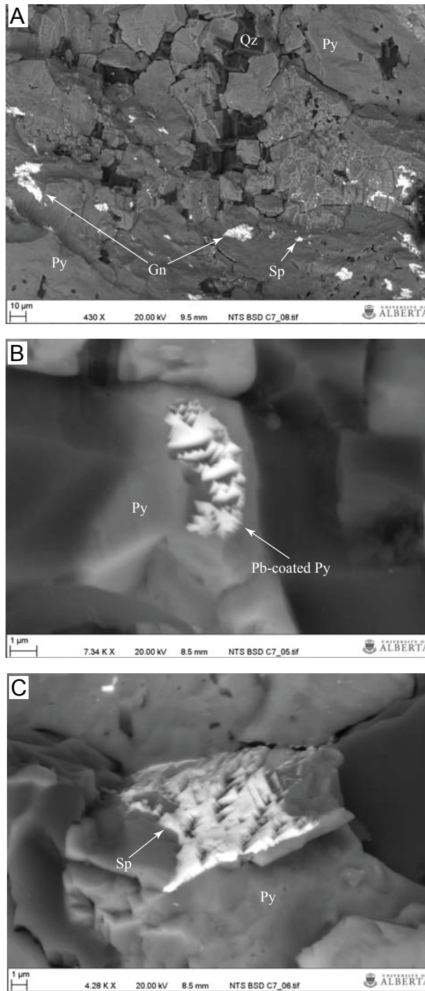
Supplementary Figure 6: SEM images show multiple episodes of re-precipitation of secondary sulfide minerals in primary pyrite mineral grains in the host rocks. (A) Anhedral secondary sulfide minerals, mainly galena (Gn) and sphalerite (Sp), both shown as high brightness in this image because of the high mean atomic mass of PbS and ZnS, completely filled the relatively large angular void spaces (a few to tens of μm) in a primary pyrite (Py) grain (grey area). The characteristics of the void spaces that host Gn and Sp are distinct from dissolution pits, which are much smaller and smoother (Supplementary Figure 5). The
