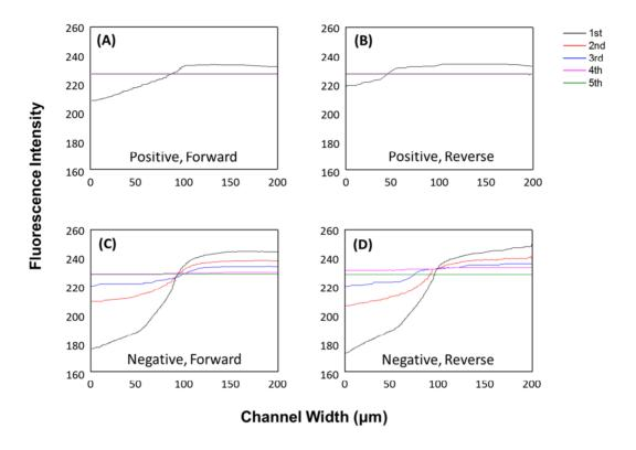
**S3** Fig. Simulated fluorescence intensity across the microchannel after each cycle. (A) Positive forward (B) Positive reverse (C) Negative forward (D) Negative reverse
