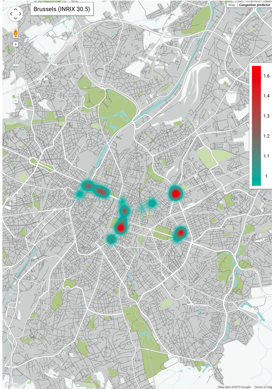
Supplementary Figure 8: Map of Brussels showing the expected ratio between incoming and outgoing vehicles of each congested junction, (\sigma_i + g_i)/d_i . Several congested junctions might appear merged in the heat map. Model parameters have been obtained assuming homogeneously distributed source and destination locations and the required road traffic to obtain an order parameter \eta [1, 2] equivalent to the city INRIX value.
