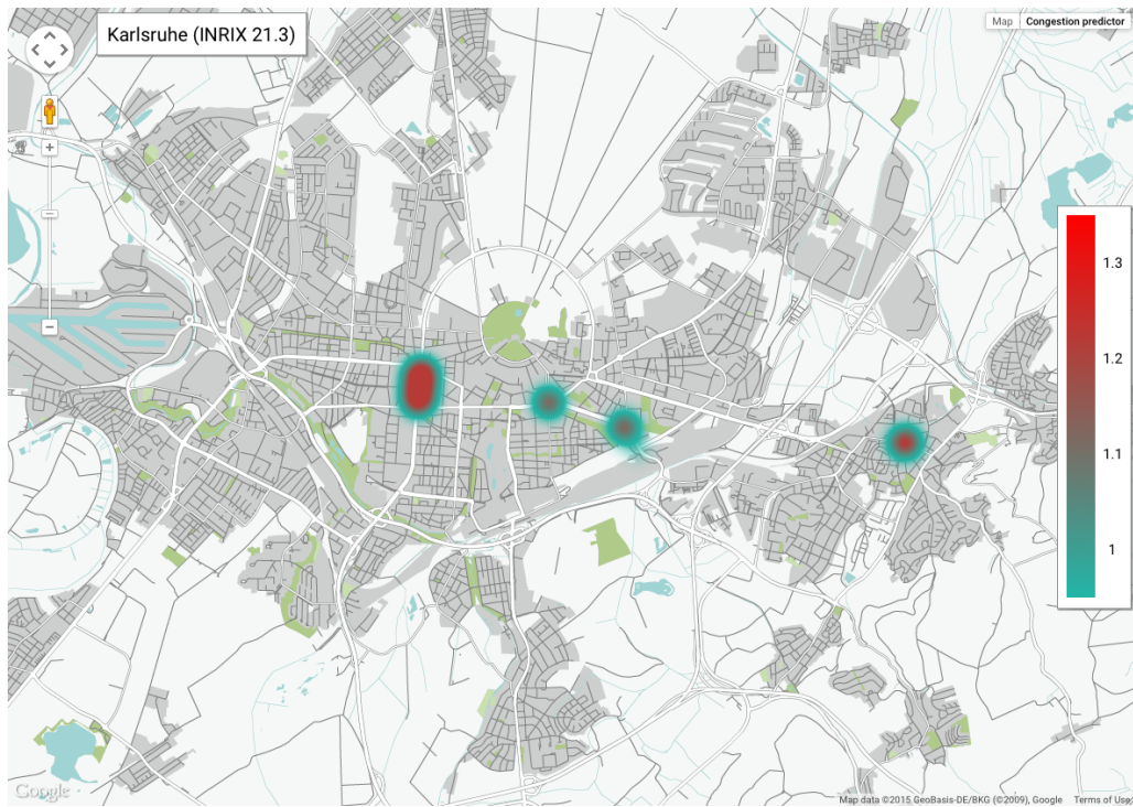
Supplementary Figure 18: Map of Karlsruhe showing the expected ratio between incoming and outgoing vehicles of each congested junction, (\sigma_i + g_i)/d_i . Several congested junctions might appear merged in the heat map. Model parameters have been obtained assuming homogeneously distributed source and destination locations and the required road traffic to obtain an order parameter \eta [1, 2] equivalent to the city INRIX value.
