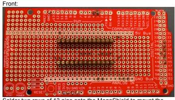
Solder two rows of 13 pins onto the MegaShield to mount the two detectors. The acrylic housing is designed for the detectors to be mounted exactly as shown.
