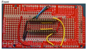
Solder a connector from AO1 to AO2 for each detector. Solder a connector from detector 1 AO2 to Arduino Analog In pin 7. Solder a connector from detector 2 AO2 to Arduino Analog In pin 5.
