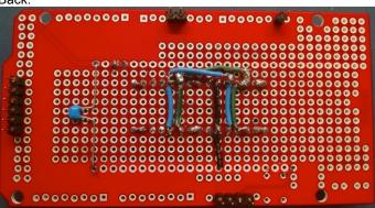
Solder connectors from CLK1 of detector 1 to CLK1 of detector 2. Solder a connector from the CLK1 to CLK2. Solder a connector from CLK2 of detector 1 to CLK2 of detector 2.
