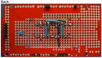
Solder analog output wires to detector pins.
