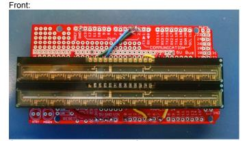
Connect detectors to pin headers. Soldering not required as heat may damage detectors. Plug in shield with detectors to Arduino Due board.
