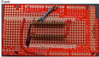
Solder a connector from Arduino PWM pin 4 to the CLK1 pin of detector 1.
