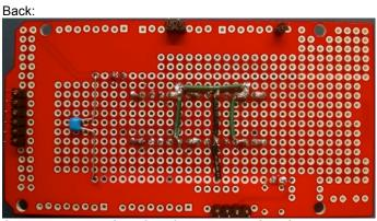
Solder connectors from SI1 of detector 1 to SI1 of detector 2. Solder a connector from the SI1 to SI2. Solder a connector from SI2 of detector 1 to SI2 of detector 2. Solder SI pins to neighboring HOLD pins
