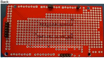
Solder pins into the power and ground. Do not solder pins into the pair of ground pins shown at the bottom right of this image or the hexagonal standoffs will not fit. Additional pins may be added for stability.
