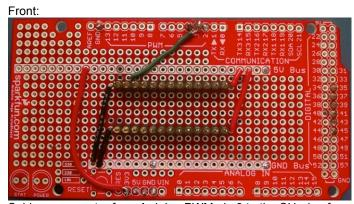
Solder a connector from Arduino PWM pin 3 to the SI1 pin of detector 1.
