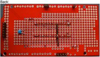
Solder the ground to the GND pins of the two detectors. Solder the 0.1  $\mu$ F bypass capacitor between the power and ground.
