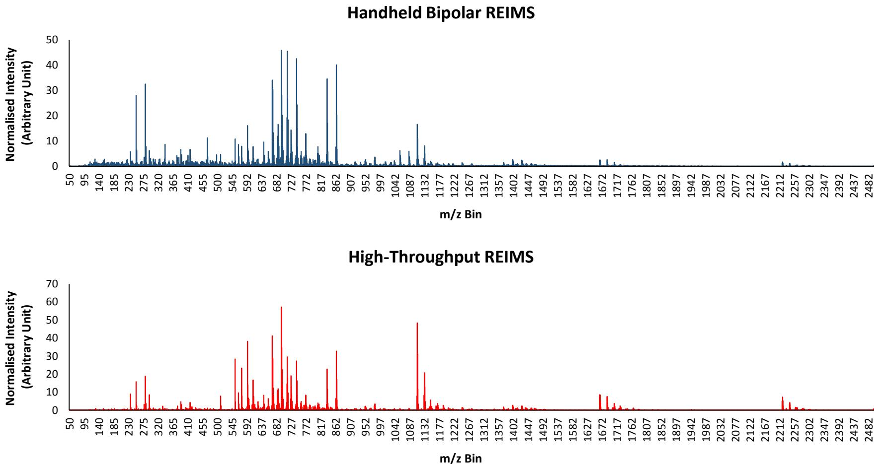
96 **Figure S3. Mean Mass Spectra of *C. guilliermondii* Isolate using Handheld Bipolar Probe and High-Throughput REIMS Approaches**
