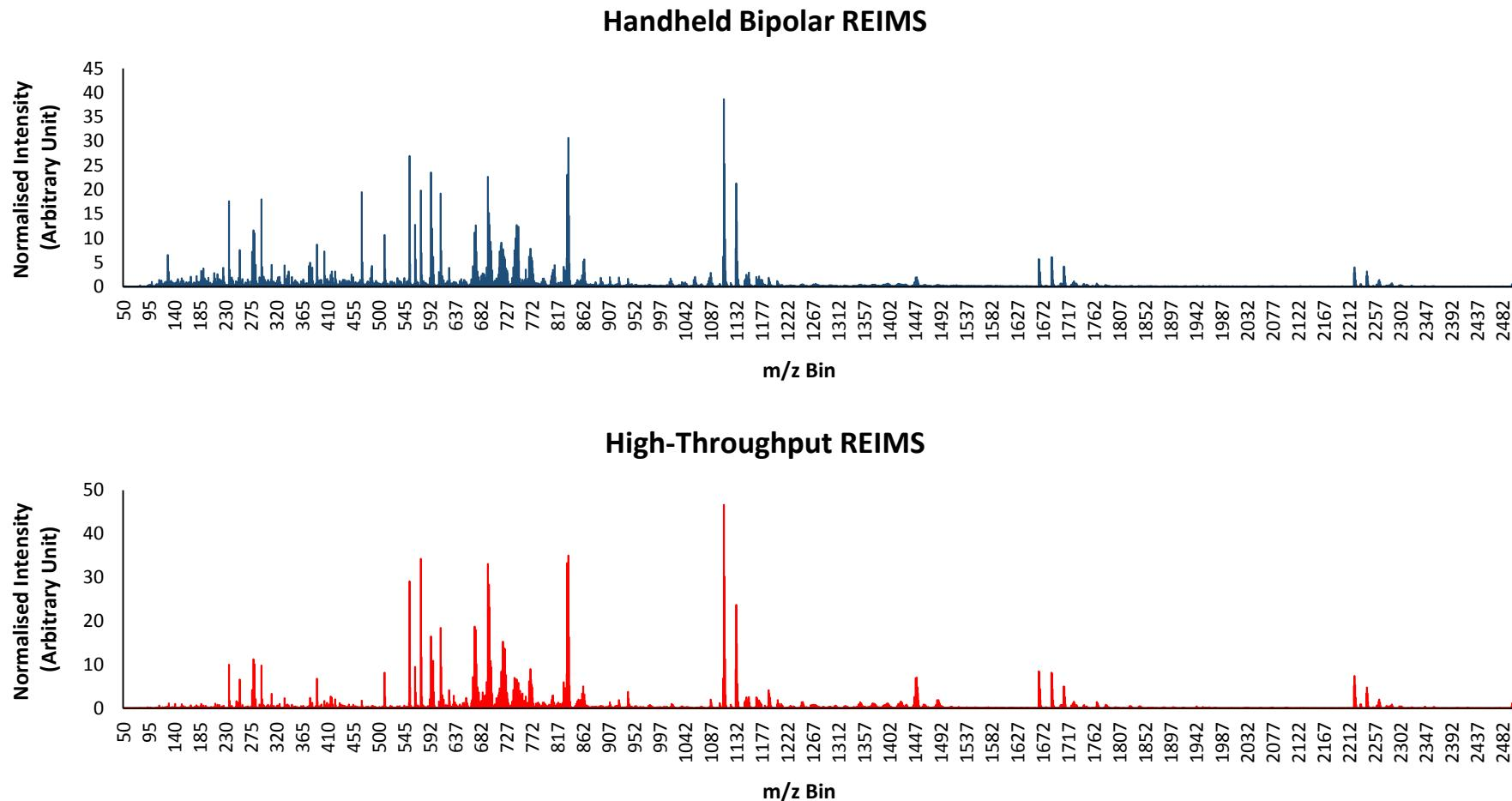
108 **Figure S7. Mean Mass Spectra of *C. parapsilosis* Isolate using Handheld Bipolar Probe and High-Throughput REIMS Approaches**
