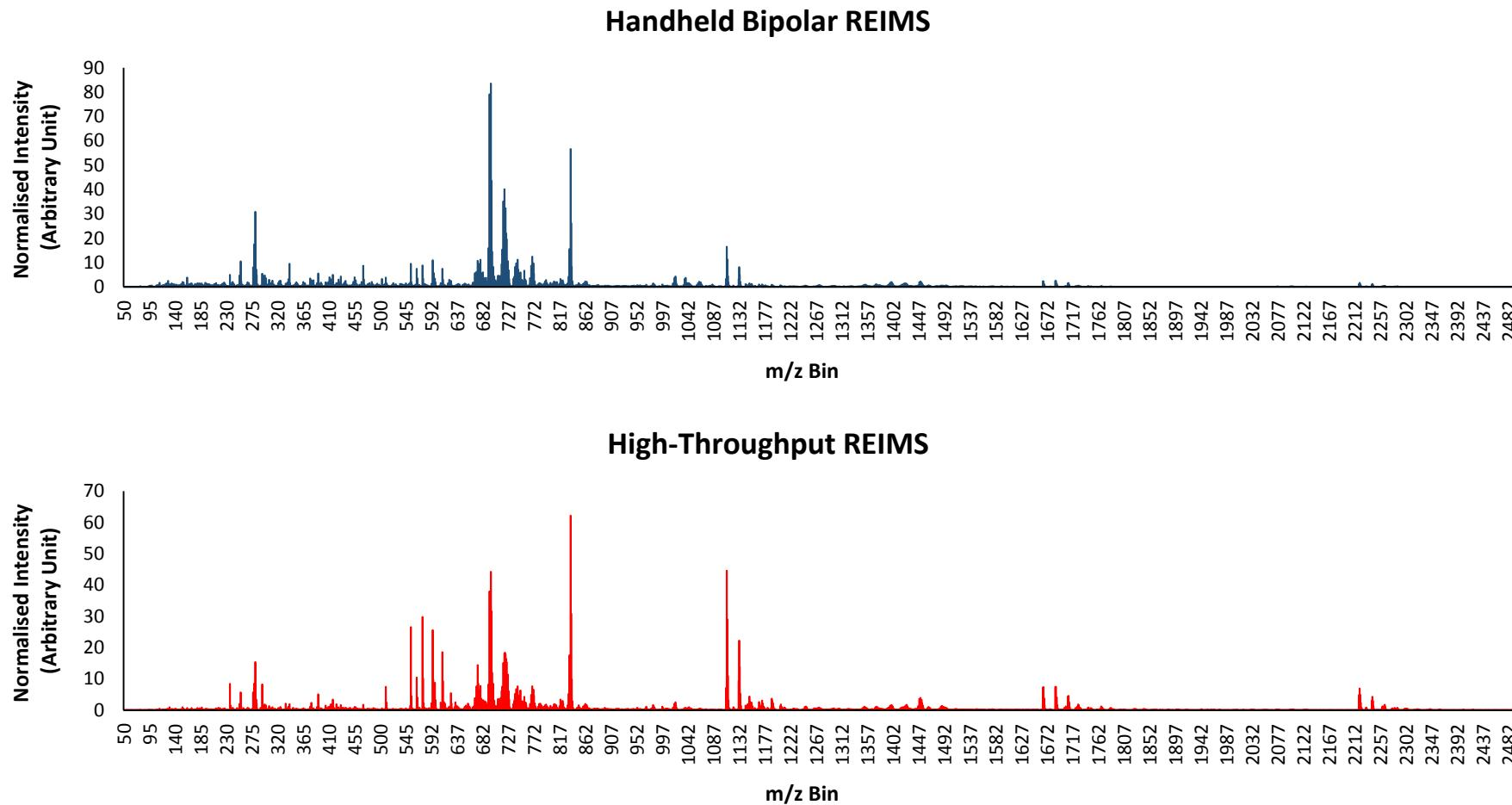
102 **Figure S5. Mean Mass Spectra of *C. krusei* Isolate using Handheld Bipolar Probe and High-Throughput REIMS Approaches**
