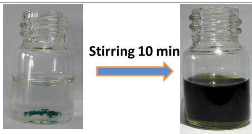
Figure S9. The change of \text{Cu}(\text{NO}_3)_3 and TBAB in 1-ethyl-2-phenylaziridine after 10 min stirring. The explorations of the solubility of copper salts ( \text{Cu}(\text{OAc})_2 , \text{Cu}(\text{NO}_3)_2 , \text{CuSO}_4 ) were carried out, and \text{Cu}(\text{NO}_3)_2 was selected as a representative to explain in details. Firstly, \text{Cu}(\text{NO}_3)_2 and TBAB were added into 1-ethyl-2-phenylaziridine. As shown in below picture, initially the solubility of copper salts was low, then, more and more copper salts were dissolved in 1-ethyl-2-phenylaziridine after stirring. Ten minutes later, solid copper salts were not observed, and the color becomes brown, indicating that copper salts have good solubility.
