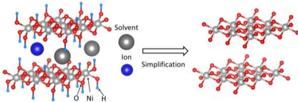
Figure S4. Illustration of simplification of NiO 2 layer structure model for Raman band assignment based on group theory.
