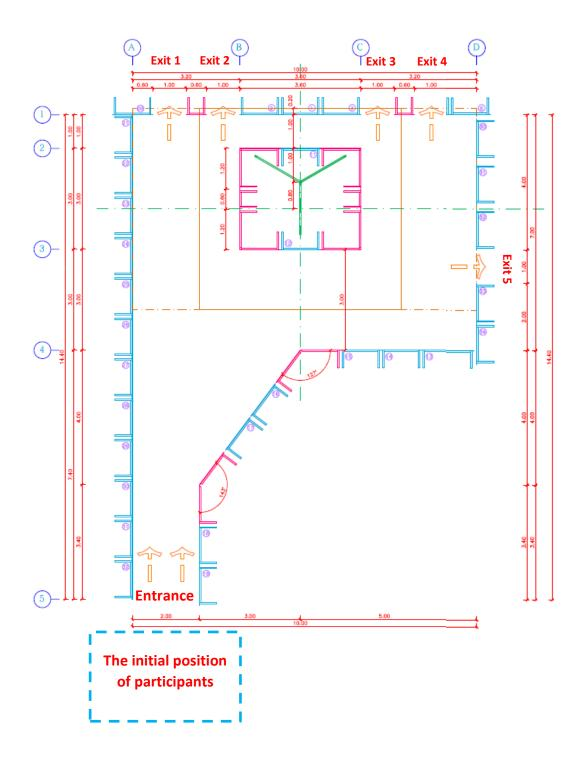
The general map of the evacuation room built for mock evacuation experiments. In total, 5 exits were built, but for each trial run only a subset of them were available to the participants. The location of the tripod legs used for mounting the camera has also been shown in green line inside the obstacle area.
