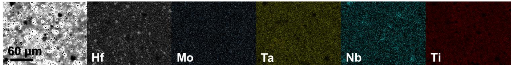
Fig. s4 Specimen #4 (\text{Hf}_{0.2}\text{Mo}_{0.2}\text{Ta}_{0.2}\text{Nb}_{0.2}\text{Ti}_{0.2})\text{B}_2 : (a) XRD patterns showing phase evolution during the HEBM-SPS fabrication process. (b) Cross-sectional SEM image and the corresponding EDX compositional maps of the specimen after SPS.
